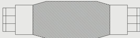
**Step 8:** Layer 3 - 1st layer of virgin rubber insulation
